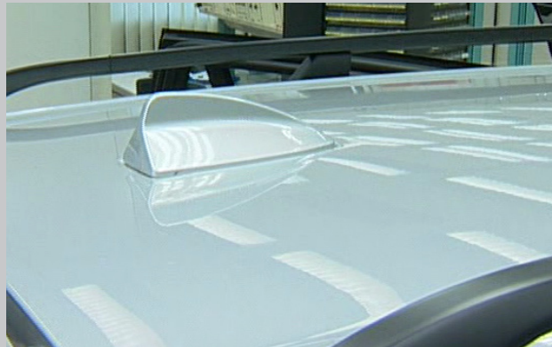
Multistandard antenna module on car roof
