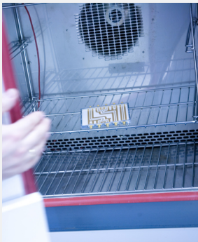
Cyclic temperature stress, e.g. even for large PCBs
