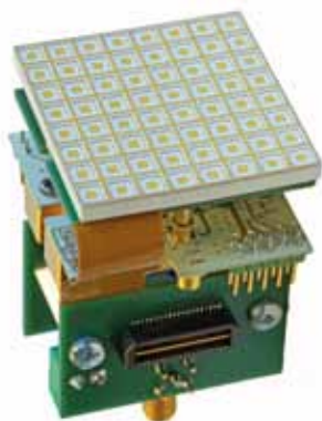
8x8 LTCC Tx-Module with integrated cooling channels
